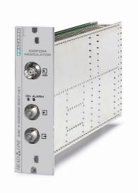
The SIG7121 modulates to DVB-T standard (using COFDM modulation) a signal received in the ASI input. It is mainly used with signals coming from an SIG7404 analogue to ASI 4 IN converter. It is possible to use up to three modulators with one receiver and are connected through the back panel.
