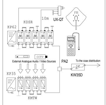
For example, it's possible to extend the existing headend by adding external analogue contents. Looking on the typical example locate on the left side, it's possible to add up to 8 different external analogue sources and mix them with 5 different satellite Free to Air contents trasmodulated into RF ouput analogue.
