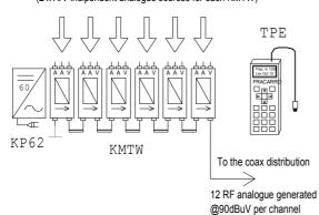
It's possible to add external analogue contents, remodulate them on RF output frequencies (SSB modulation – Standard BG-Pal).
