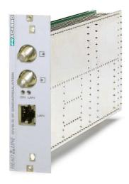
The SIG7710 is an Encoder that works as a DVB-S to IP gateway. Satellite signals are received on the F connector input, converted to IP standard signals and streamed through RJ45 output port into LAN.
