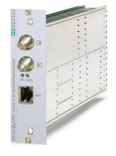
The SIG7730 is an Encoder that works as a DVB-T to IP gateway. Digital Terrestrial Television (DTT) signals are received on the F connector input, converted to IP standard signals and streamed through RJ45 output port into LAN.
