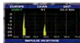
Impulse response (ECHO in COFDM TV)
