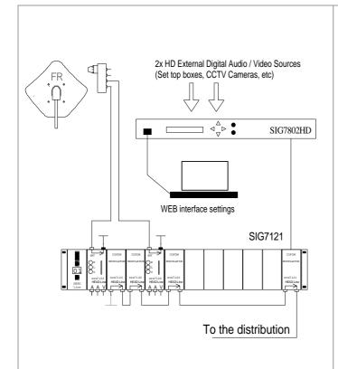
It's possible to use the HEADLine architecture and mix some HD contents in the coaxial network by using the new professional SIG7802HD encoder coupled with a SIG7121 digital HEADLine modulator.
