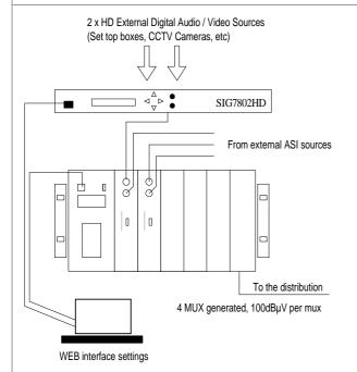
The SIG7802HD can encode up to two different HD digital sources, for example HD CCTV cameras, FTA set-top-boxes, and so on.
