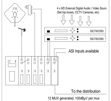
The 3DGFlex architecture allows the installer to create a mixed configuration in which it is possible to distribute the SD or HD programs received from the satellite dish, from the aerials as well as many HD auxiliary content previously "encoded" by the digital external professional encoders (see example on the left side).
